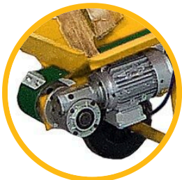
230V electric Reduction gearbox
